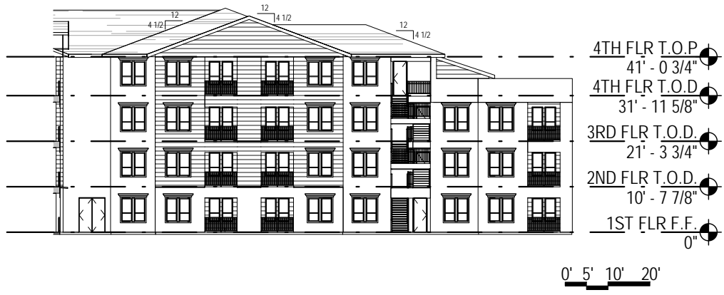
② BUILDING A - WEST ELEVATION 1/32" = 1'-0"
